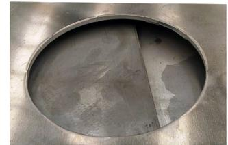
**Hole Punched with Tri-Radius**
