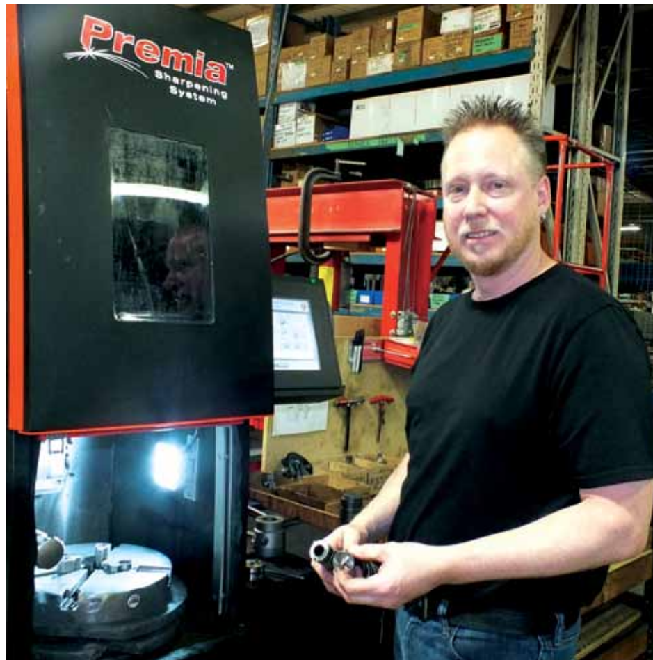
Vince Scott holding the Mate punch tooling beside an earlier investment Laicor made two years ago on a Mate Premia sharpening system, which works for dies, punches and inserts.
