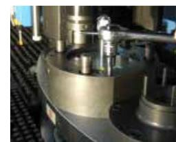
Photo 6: Tighten the upper and lower tool holder retaining screws.
