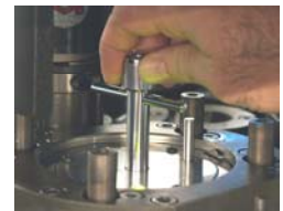
Photo 2: Tighten tensioning knob on adjustment handle until knob starts to click.
