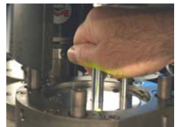
Photo 4: Align the station, using the T-bar to tighten the adjustment handle until the light goes green.
