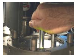
Photo 5: Align the station, using the T-bar to tighten the adjustment handle until the light goes green.
