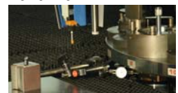
Photo 5: Draw the probe of the dial-test-indicator along the length of the alignment bar.
