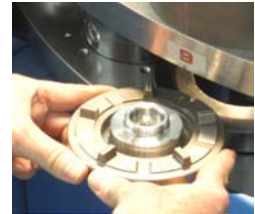
Photo 2: Install Lower Instrument
