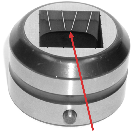
Photo 1: Mate Slug Free Light notches are cut at an angle to create a series of protrusions on the slug. As the slug moves through the die, the protrusions become trapped against the die land to prevent the slug pulling back on to the sheet. (Image enhanced for additional clarity)
